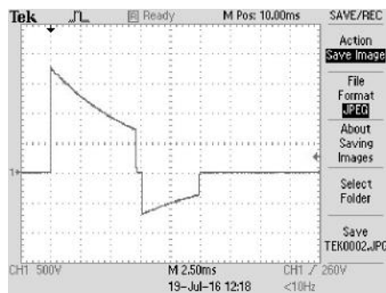
Defibtech Adult waveform at 75 ohms
